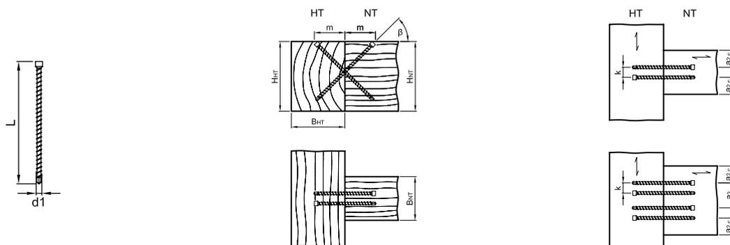
$a_2 = \text{min. } 40 \text{ mm}, a_{21} = \text{min. } 24 \text{ mm}, k = \text{min. } 12 \text{ mm}$
