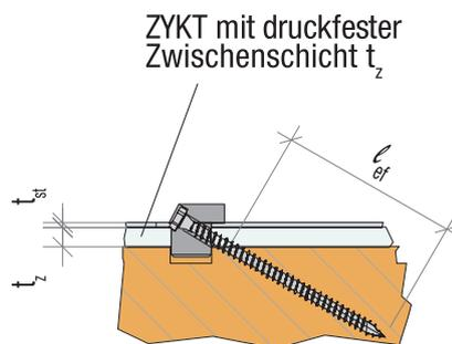
$$l_{ef} = l - (t_{st} + t_z) \times 2$$
