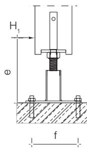
$$R_{\text{axial,Bolzen}} = \frac{H \times e}{f}$$
